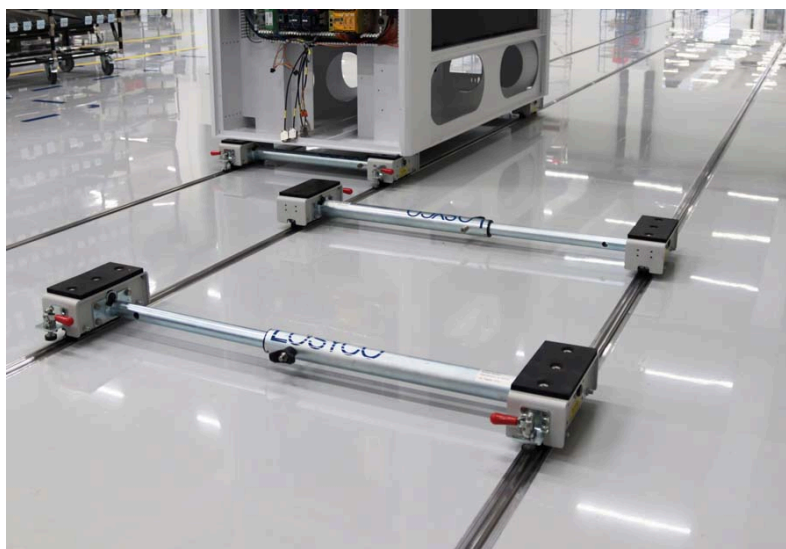
Caption 1: Assembly line for wire bonders: variable conveyor concept with customer-specific transport trolleys for different track spacing
