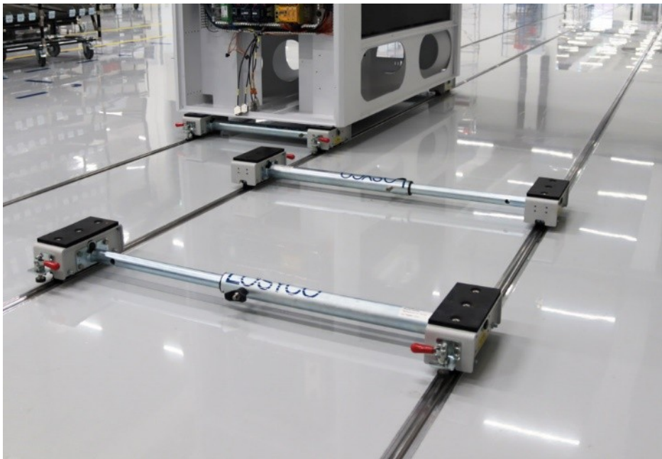
Caption: LOS YCO has tailored trolleys with telescopic axes for intra-logistics transport on LOXrail tracks with different widths
